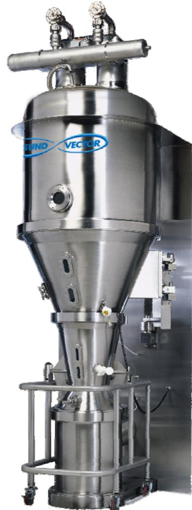
*VFC-30MX Shown with Bottom Spray Tapered Wurster Insert*
